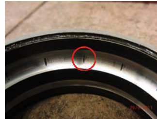
Without micro-pulsing Depth approx. 0.08 mm
